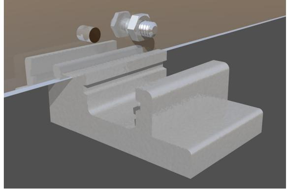
**Step 3c**-Mount a fastener at each end of the mirror. Place corner of the mirror in the middle of fastener so that half of the fastener extends beyond the mirror.
