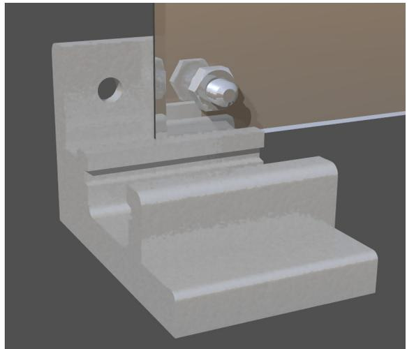
**Step 3d**-Arrange the fasteners so they are flat and straight centered along the rail. The right-most fastener will mount where you have marked the center of the rail in step 2.
