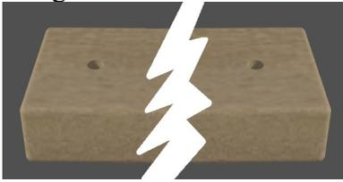
**Step 2**-Mark the center-point of the rail with a pencil on the 2" side of rail that will ultimately face downwards. The four mirrors will be arranged in a single series along the middle of the support. For the purpose of this discussion, mirrors are numbered from left to right as 1, 2, 3 and 4. This procedure describes how to mount them in a chronologic order of 2, 3, 1, 4. You will mount them with the reflective side of the mirror facing you and the back side away from you.
