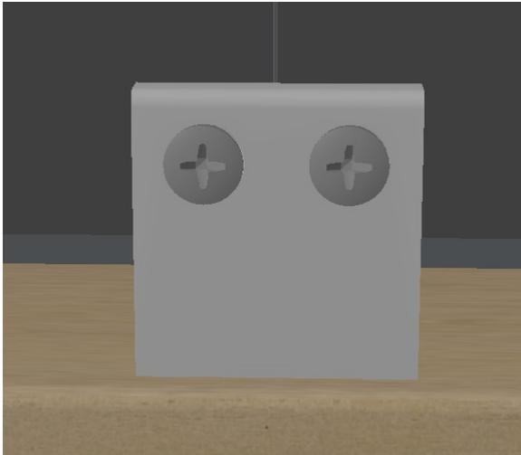
**Step 5**-Prepare Mirror 1 in similar fashion to the procedure for step 4. The fastener that goes on the left end will also be at the left end of the whole series. For Mirror 1 & 4, the fastener that is not shared should be mounted so that its outer edge is flush with the end of the mirror. The other hole in the fastener will go unused.
