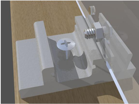
**Step 4**-Prepare Mirror 3 in similar fashion to procedure for the first mirror in steps 3a~3f. You will only need two fasteners and two wood screws. One goes in the middle of the mirror and the other goes on the right end. The left end will share the right fastener of Mirror 2 that is in the center of the rail. After mounting the Mirror 3 assembly, the back side of the joining fastener should look like the picture below. This view is from the non-reflective side of the mirrors.
