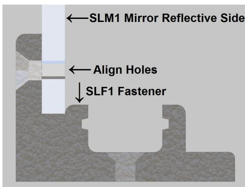
**Step 3b**-Insert a machine screw to one of the dual counter-sunk holes on the back of fastener and secure it through the mirror with a nut. It doesn't matter which hole you use.
