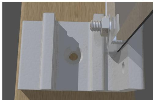
**Step 3f**-Secure the assembly to the rail with three supplied wood screws.
