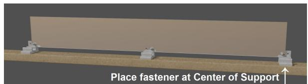
**Step 3e**-Mark the position of the hole in base of each fastener with a pencil. Then drill three pilot holes in the rail with a 1/16" drill bit.
