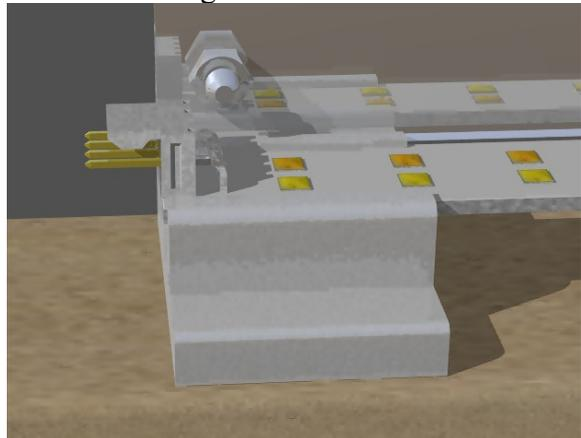
**Step 8**-Repeat this process for each of the modules until they are all mounted. Be careful to seat the male connector into the preceding modules's female connector as you thread it back through its fastener.
