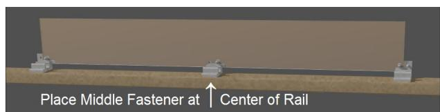
**Step 3e**-Mark the position of the hole in base of each fastener with a pencil. Then drill three pilot holes in the rail with a 1/16" drill bit.
