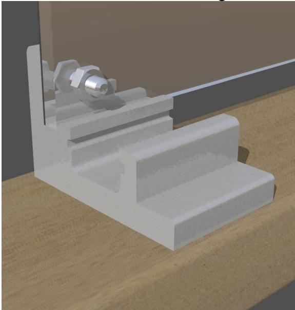
After mounting the Mirror 1 assembly, the back side of the joining fastener should look like the picture below. This view is from the non-reflective side of the mirrors.
