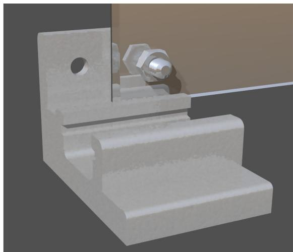
**Step 3d**-Arrange the fasteners so they are flat and straight centered along the rail. The fastener in the middle of the mirror will mount where you have marked the center of the rail in step 2.
