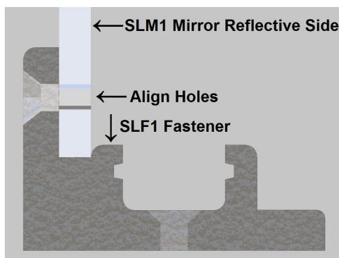
**Step 3b**-Insert a machine screw to one of the dual counter-sunk holes on the back of fastener and secure it through the mirror with a nut. It doesn't matter which hole you use.
