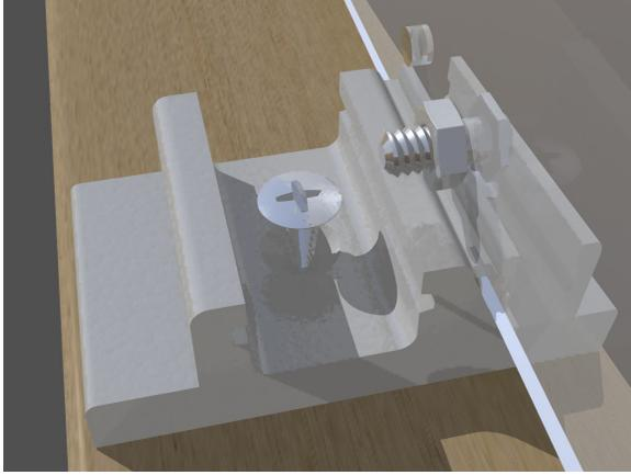
**Step 4**-Prepare Mirror 1 in similar fashion to the procedure for steps 3a~3f. The fastener that goes on the left end will also be at the left end of the whole series. For Mirror 1 & 3, the fastener that is not shared should be mounted so that its outer edge is flush with the end of the mirror. The other hole in the fastener will go unused.
